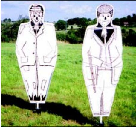
Each of the two scarecrows comprises a human profile made out of tough reinforced long life PVC which is stretched over an easily assembled steel and aluminium frame to create an S shaped aerofoil which has a screen printed human figure on one side and is predominantly white on the reverse side. This revolves on good quality bearings in the slightest breath of wind, with the whole body being held securely upright, even in the strongest winds, on a metal fencing spike.
